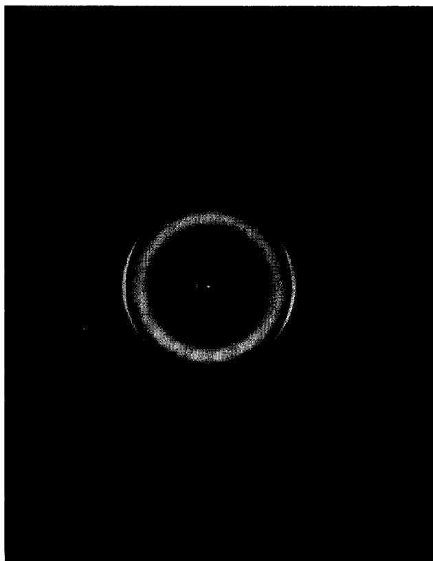
Figure 7 Wide-angle X-ray diffraction pattern of a paraffin oil-containing polyethylene fibre stretched in the spinline. The fibre was spun at T_{\text{spin}} = 170^\circ\text{C} and a speed of 100 m/min. The take-up speed was 400 m/min
