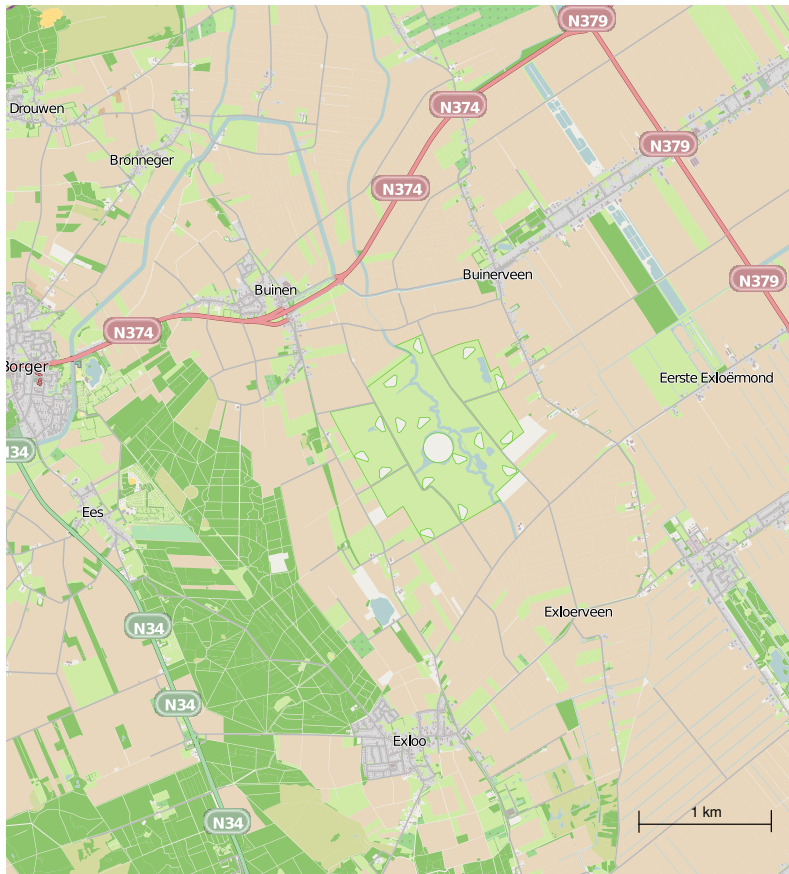
Figure 1.3: Map of the LOFAR core and its surroundings. The circular peninsula in the centre is the Superterp. Several other stations are visible as well. (source: OpenStreetMap)
