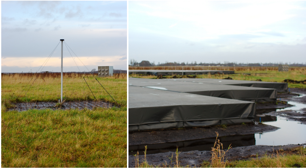
Figure 1.2: Antenna types of the Low-Frequency Array. Left image: A low-band antenna with a cabin in the background. Right image: Part of a high-band antenna station, consisting of 24 tiles of 4 \times 4 high-band antennae.
