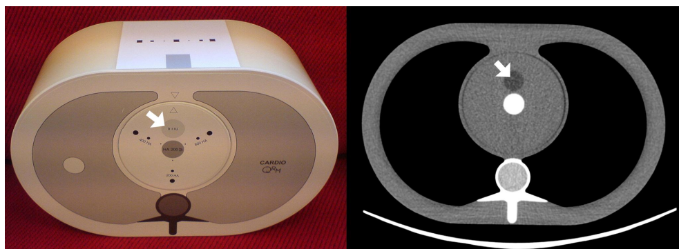
Figure 3-3. The photograph (left) and CT image (right) of the thorax phantom.
