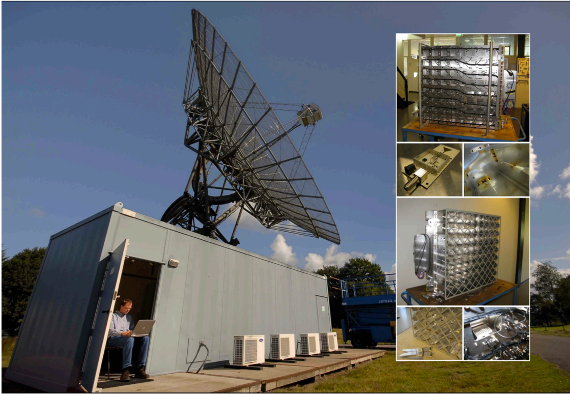
Figure 1. The WSRT telescope RT5 equipped with the APERTIF prototype. Shown in the inserts is the Vivaldi array in the lab
