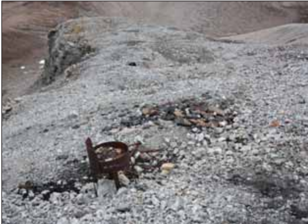
4.28 Small furnace, mining tools, and stockpile of iron ore below the mine on Iron Mountain. (Photo: C. Botman, LASHIPA 9, 2010.)
