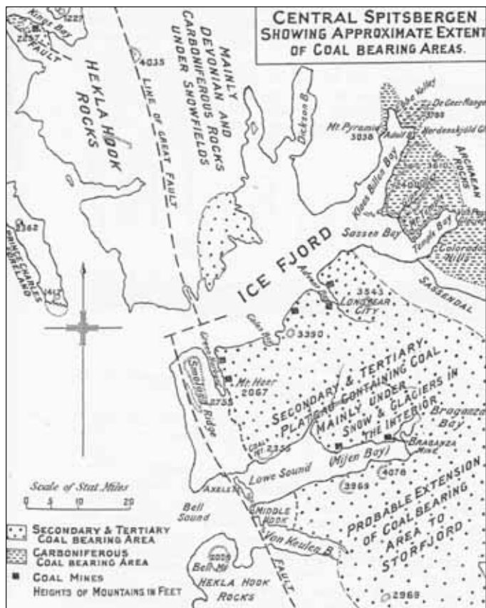
8.20 Map showing Spitsbergen's coalfields. Note that the working mines were confined to the Tertiary deposits. (Source: Cadell, H. M. (1921) 'Coal-mining in Spitsbergen', Transactions of the Institution of Mining Engineers , 60, 119-42.)
