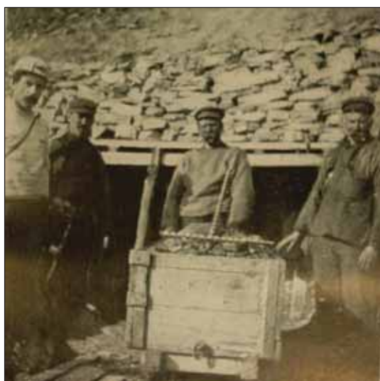
6.10 Wooden tubs used in a mine at Camp Morton. Note Ernest Mansfield in the light jumper on the far left. (Source: The Northern Exploration Co., Ltd. (1911) The Northern Exploration Company, Norwegian Polar Institute, Tromsø, p. 94. )
