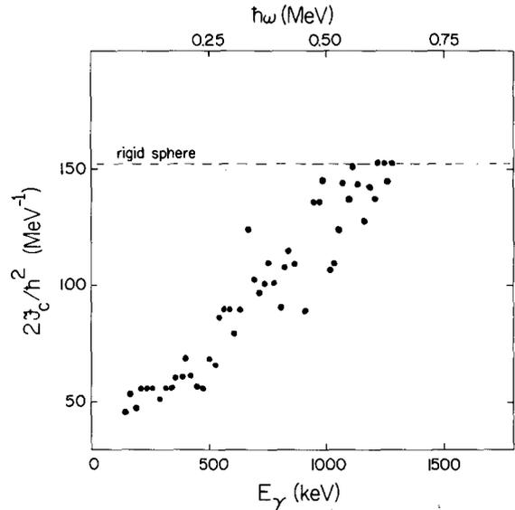
Fig. 3. The derived collective moment of inertia plotted as a function of  $\gamma$ -ray energy and of rotational frequency ( $\hbar\omega \approx \frac{1}{2}E_\gamma$ ). The fluctuations in  $2\mathcal{I}_c/\hbar^2$  are probably due to experimental uncertainties.
