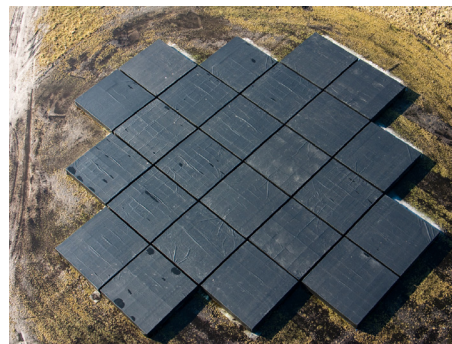
Fig. 1. Twenty-four-tile HBA station. Each tile is one station element. This is the station configuration for most of LOFAR's HBA stations, including the LOFAR core (CS302). It is clear that a station like this is highly redundant.
