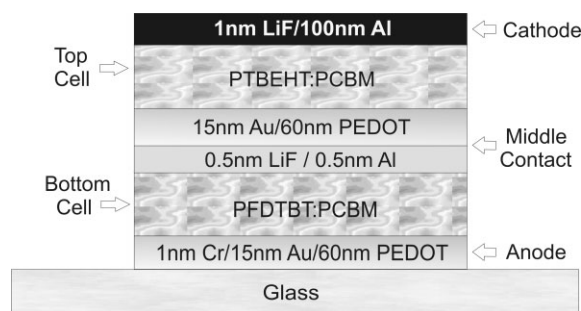
Figure 8. The structure of a solution-processed tandem organic solar cell as processed in Ref. [43]. The two bulk heterojunction sub-cells are connected in series by the semitransparent middle contact. The absorptions of the sub-cells are complementary.
