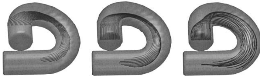
Figure 12. Streamlines starting on a horizontal plane, for Re = 1 (left), Re = 10 (middle) and Re = 100 (right).
