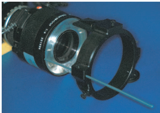
Figure 4. The custom made snap-on ring for the extension bar on the camera lens. The ring is placed over the lens.
