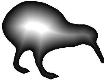
Fig. 1. The distance transform of an object. The pixel intensity denotes distance to the object boundary.
