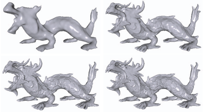
Fig. 3. Example of reconstruction at various octree depths: Top-left : D = 7 , top-right : D = 8 , bottom-left : D = 9 , bottom-right : D = 10 .
