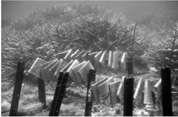
Fig. 9. Terracotta tiles with custom holobionts placed at a field location where Acropora spp. are common.
