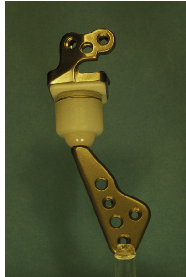
Fig. 1. Groningen TMJ prosthesis consisting of a mandibular part, an intervening disc and a cranial part. The cranial part consists of a fitting member and a basic part. In lateral view.
