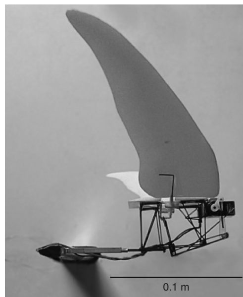
Figure 1: Flapping-wing MAV mounted on the force balance. Wing-span = 0.33 m, average chord length = 40 mm, aspect ratio = 8.3.
