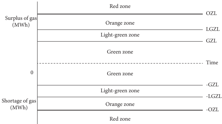
Figure 2. Different degrees of network imbalance
