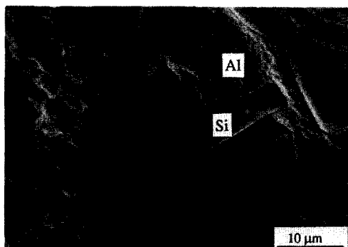
Fig. 1. The surface of the Al drop after reaction contains many Si precipitates, which may prohibit the formation of a spherical shape of the liquid drop.
