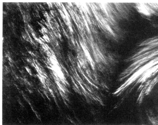
Figure 8. Polarized optical microscopy picture of a 60/40 (w/w) \text{P4VP}(\text{DBSA})_{1.0} /xylene sample at room temperature sheared by sliding the cover slip.
