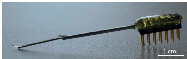
Figure 3.16: Illustration of the packaging used for acute experiments in rats.
