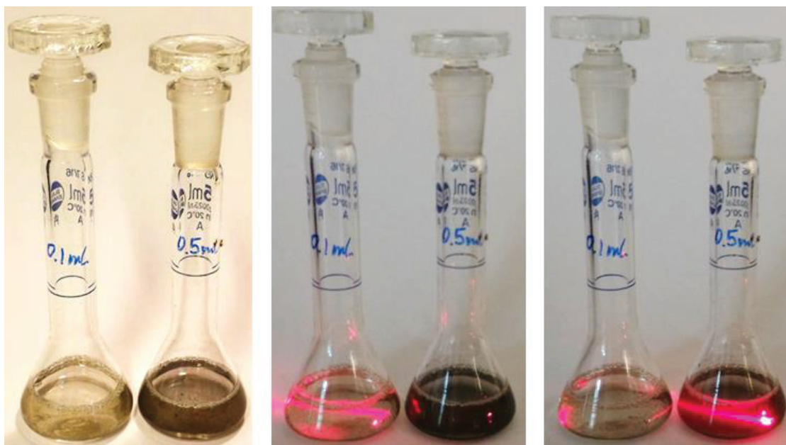
Figure 9.5. Dramatic change of colloidosome solution color with increasing AuNPs content by 5 times. On the left, colloidosomes obtained from one monolayer of initial nanoparticles surface coverage; on the right – from 5 monolayers.
