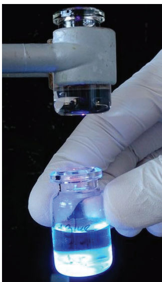
Figure 9.8. Ongoing UV-curing process. Bright blue phase at the bottom of the flask is DCE with polymer glue covered by 1/8 monolayer (ML) of nanoparticles.
