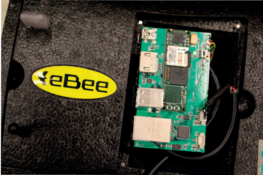
Figure A.3: Hardware setup consists of Gumstix Linux microcomputer and extension board which has an access to the autopilot data and Gumstix ports.
