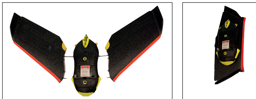
Figure A.2: Ebee platform, wings can be detached from the main body and it can be folded for easy transport.
