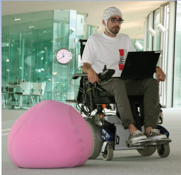
Figure 2. A brain-controlled wheelchair: users can drive it reliably and safely over long periods of time thanks to the incorporation of shared-control (or context-awareness) techniques.
