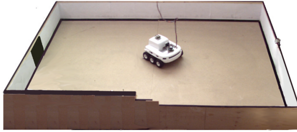
Figure 8: A mobile robot Koala equipped with a vision module gains fitness by staying near the lamp (right side) only when the light is on. The light is normally off, but it can be switched on if the robot passes near the black stripe (left side) positioned on the other side of the arena. Position of the robot is controlled by an external positioning system and passed to the computer in order to control the light and to compute the fitness.
