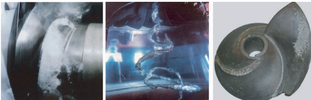
Figure 3: Typical developed cavitation on rotating inducer (left), cavitation vortex rope downstream a Francis turbine (center), cavitation erosion on pump impeller (right).
