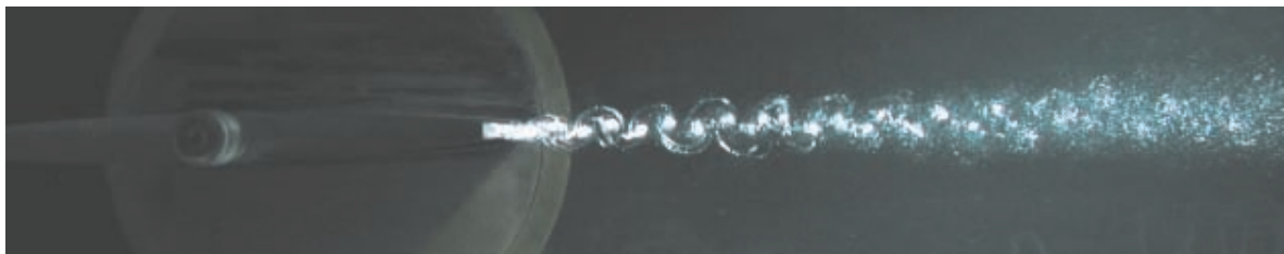
Figure 7.1: Shedding of Von-Kàrmàn street on NACA0009 hydrofoil [13]
