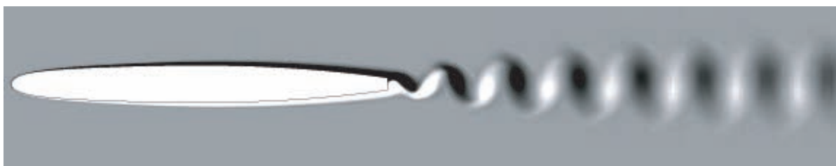
Figure 7.3: Computed spanwise vorticity (Von-Kàrmàn street) on NACA0009 hydrofoil positive : black, negative : white, C_{ref}=20\text{m/s} , i=0^\circ , cavitation free regime
