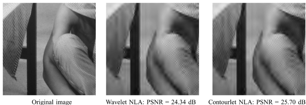
Fig. 16. Nonlinear approximation by the wavelet and contourlet transforms. In each case, the original image Barbara of size 512 \times 512 is reconstructed from the 4096-most significant coefficients. Only part of images are shown for detail comparison.
