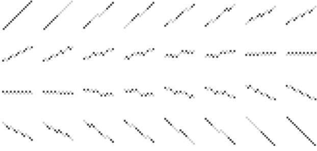
Fig. 6. Impulse responses of 32 equivalent filters for the first half channels, corresponding to the mostly horizontal directions, of a six-level DFB that uses the Haar filters. Black and gray squares correspond to +1 and -1, respectively. Because the basis functions resemble “local lines,” we call them Radonlets .
