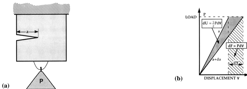
Figure A-1. Graphical definition of the strain energy release rate, for a structure in load control. (a): crack plate subjected to a fixed load, P ; (b): load-displacement response of the plate for a crack of length a and a+da . dU is the strain energy release rate. From [3].
