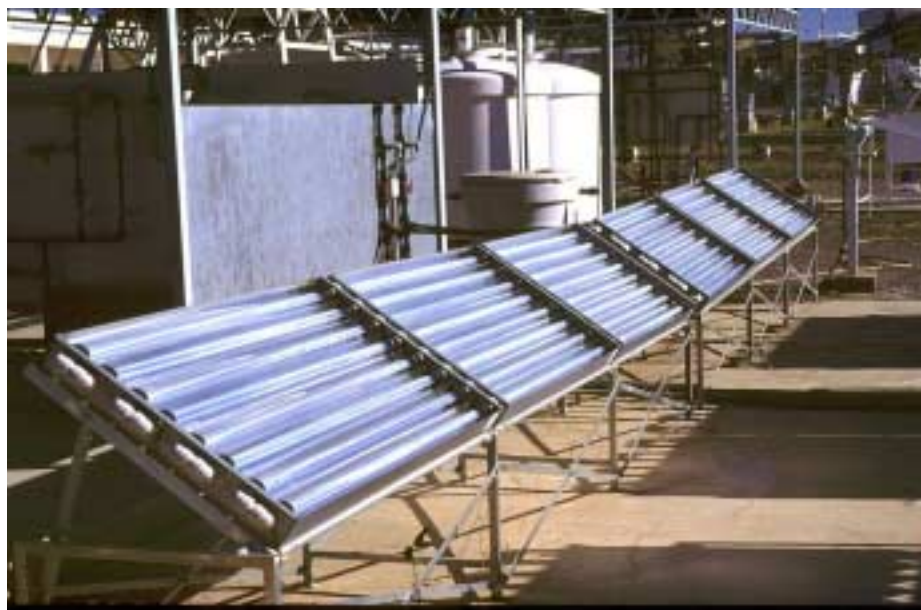
FIGURE 4.10 View of the CPC used for the solar driven experiments at the PSA.
