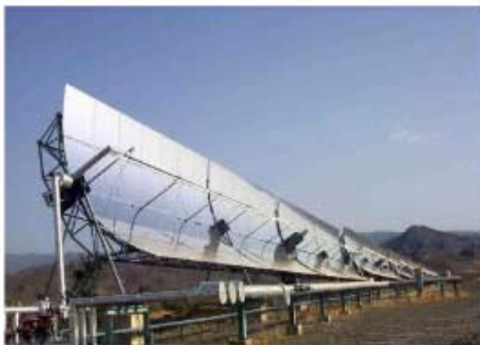
FIGURE 4.5 Medium-concentrating solar collectors. PTC type (PSA, Spain).
