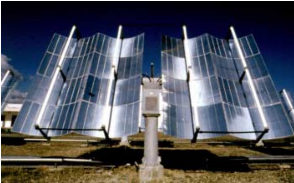
FIGURE 4.9 HM-type collector in tracking position.
