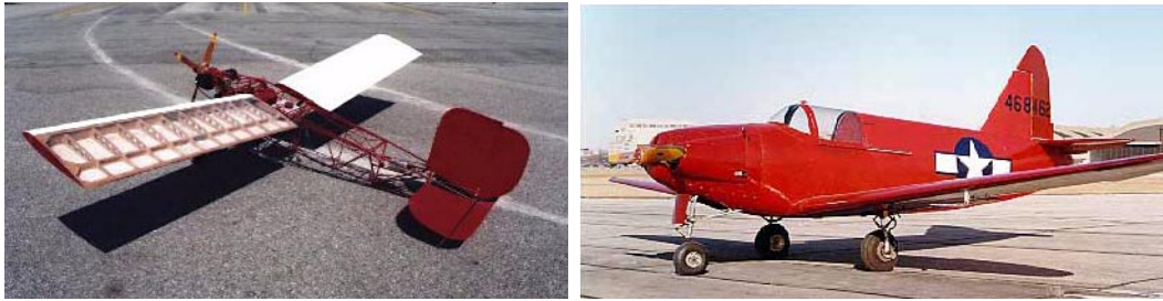
Figure 43. Radio-controlled target drones: left , Radioplane RP-5A (Western Museum of Flight); right , Culver PQ-14 Cadet (USAF Museum).
