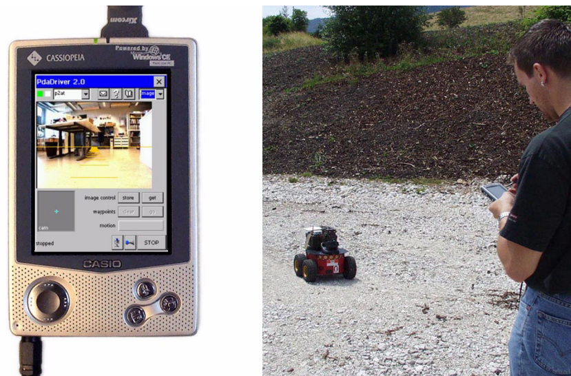
Figure 12. Left, PdaDriver; right, field-work with PdaDriver.
