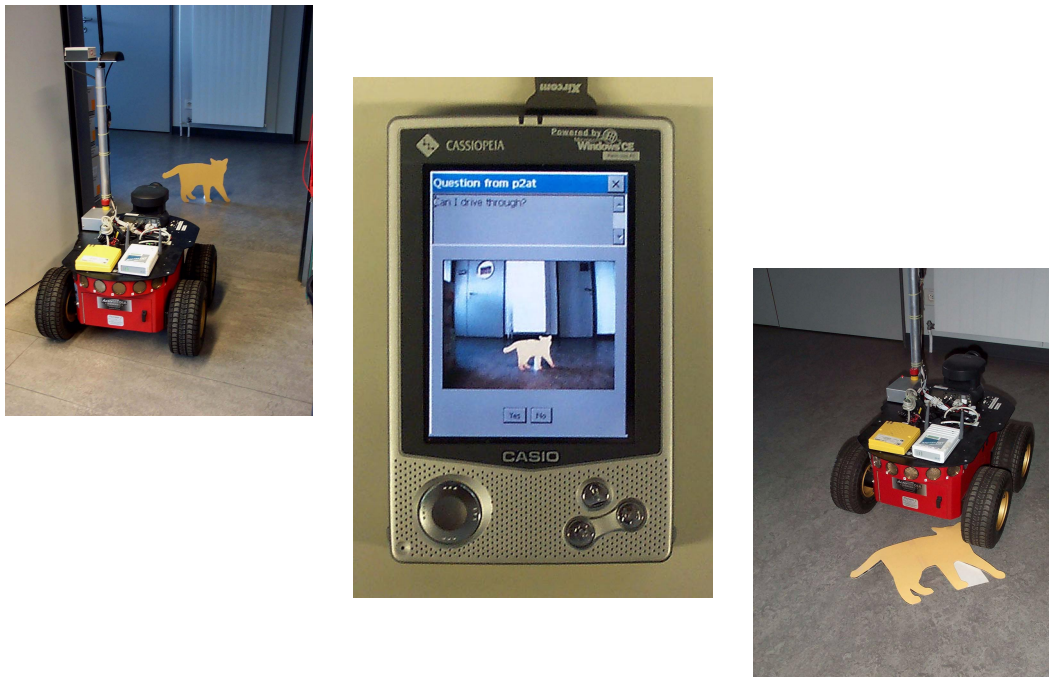
Figure 1. Vehicle teleoperation using collaborative control: Left , robot encounters a potential obstacle; center , query to the human: “Can I drive through?”; right , collaboration result.
