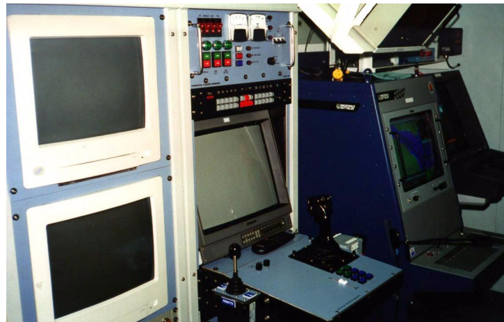
Figure 51. Direct teleoperation interface (International Submarine Engineering, Ltd.)
