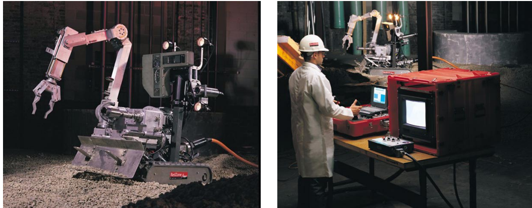
Figure 47. Left , the Pioneer robot; right , Pioneer control console. (Carnegie Mellon University and RedZone Robotics, Inc.)
