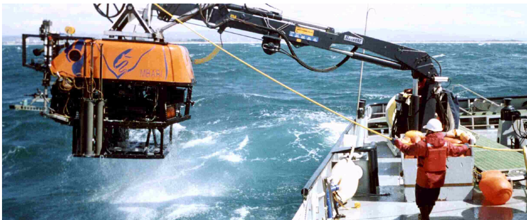
Figure 50. A work-class ROV designed for drilling support and oceanographic research (International Submarine Engineering, Ltd.)
