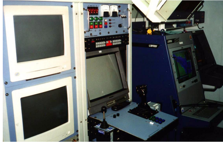
Figure 3. Direct teleoperation interface (International Submarine Engineering, Ltd.)
