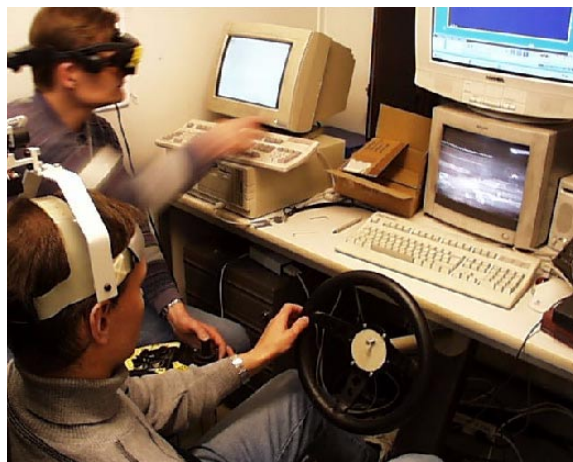
Figure 52. Telepresence interface for heavy work vehicles (Helsinki University of Technology)
