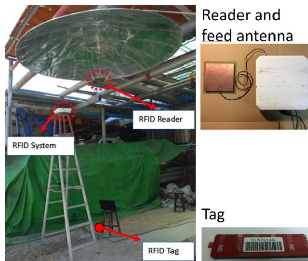
Fig. 8. Measurement setup with the RFID system equipped with the ellipsoidal reflector reader antenna.
