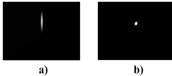
Figure 6: (a): The beam spot of the reference beam I on polarizer P_A in conditions of moderate sunlight and with feedback OFF . (b): The same spot with feedback ON . The diameter of the circular spot in 6b) is 0.3 mm.
