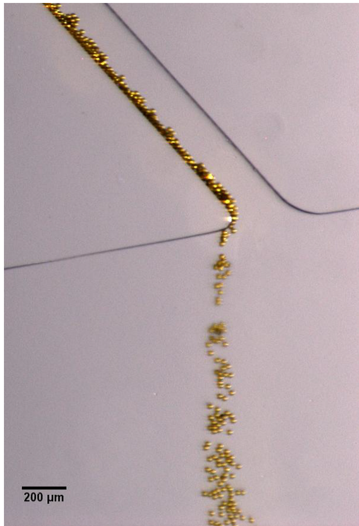
Figure 7.6: Routing of isolated yellow beads to the capture chamber with a purity of 99%.
