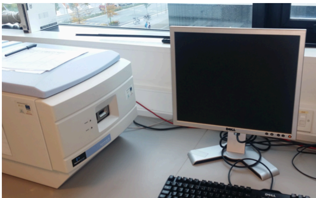
Figure 1.22 Photograph of Perkin Elmer Scan array Gx Microarray scanner, fluorescence scanner set
