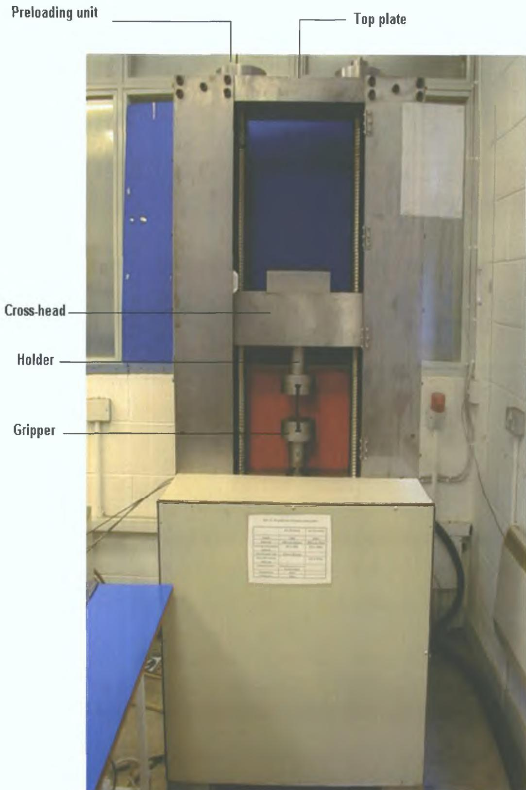
Plate 3.1 Torque-tension machine
