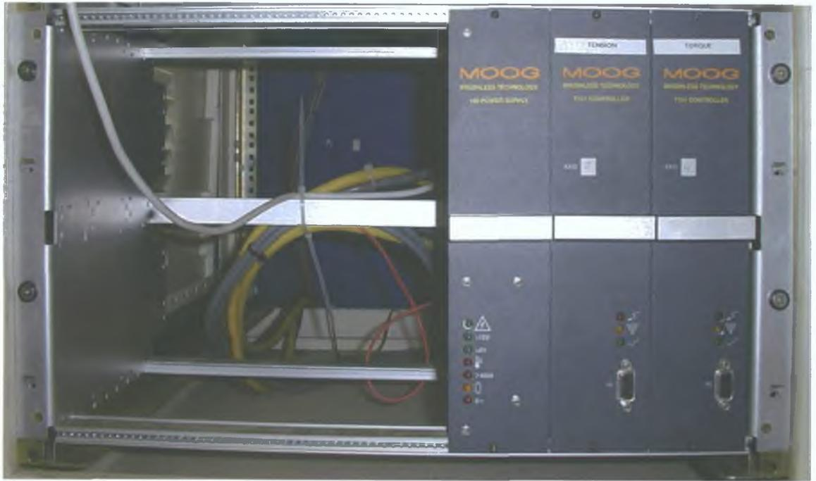
Plate 3.4 The two identical "Moog T161-003" brushless motor controllers
