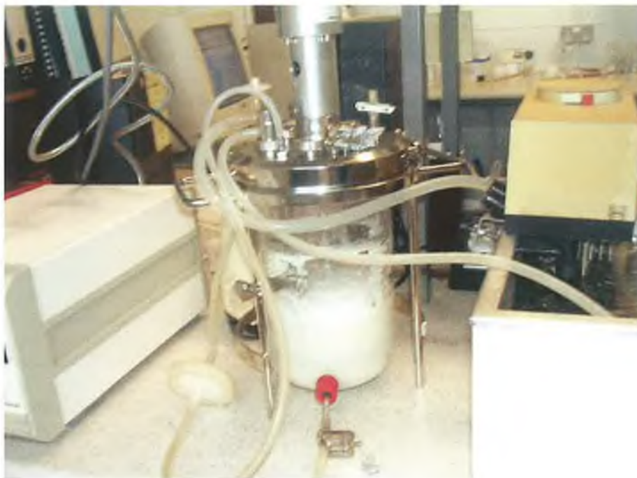
Figure 3.3.4: Illustration of the 2 L fermenter set-up after 24 h growth of Y. lipolytica RP2 on tallow ( 20 \text{ g L}^{-1} ) with pH control to pH 7.0 by 0.1 M potassium phosphate buffer. Agitation and aeration were set at 500 rpm and 1 vvm, respectively. Temperature was controlled to 25^\circ\text{C} by a circulating water bath.
