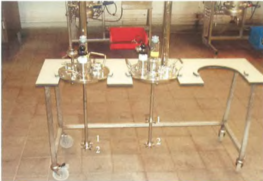
Figure 3.3.10: Illustration of the impeller position on the agitator for the 10 L fermenter. (A) 2 impellers are positioned at the base of the shaft and (B) 1 impeller is positioned at the base of the shaft with the second impeller 135 mm above it.
