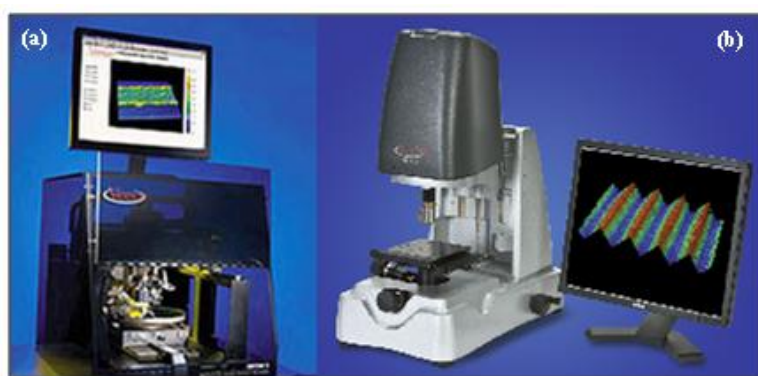
Figure 37: (a) the Veeco Detak 8 Profiler, (b) the Veeco NT9080™ Surface Metrology System
