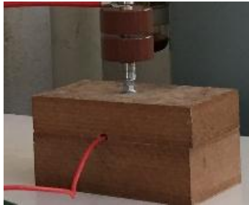
Figure 4. 3 The coupling capacitor
