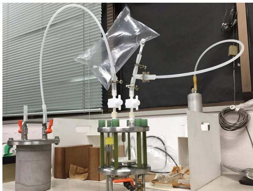
Figure 4. 7 Schematic diagram of oil filling process.
