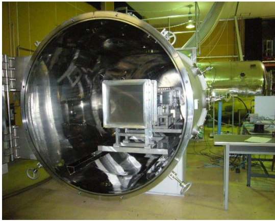
(a) Mars Wind Tunnel in Vacuum Chamber
