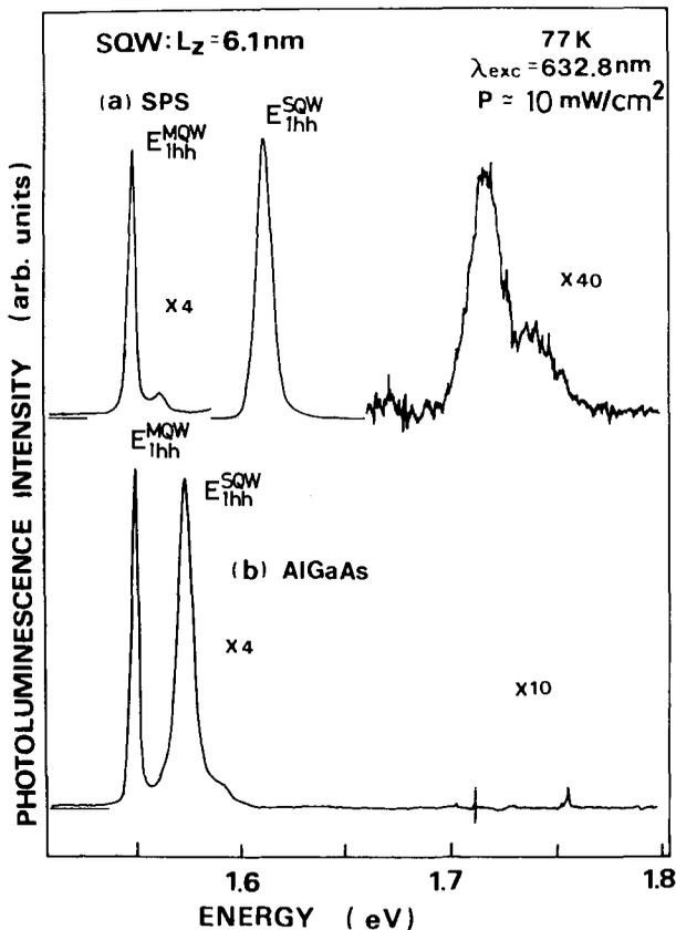
FIG. 1. 77 K photoluminescence spectra of two types of SQWH samples with (a) GaAs/AlAs SPS's and (b)  $\text{Al}_{0.24}\text{Ga}_{0.76}\text{As}$  cladding layers both with MQW buffer.
