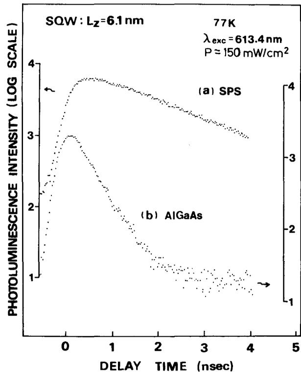
FIG. 2. Decay of the SQW photoluminescence intensity for two types of SQWH samples with (a) GaAs/AlAs SPS's and (b)  $\text{Al}_{0.24}\text{Ga}_{0.76}\text{As}$  cladding layers both with MQW buffer.
