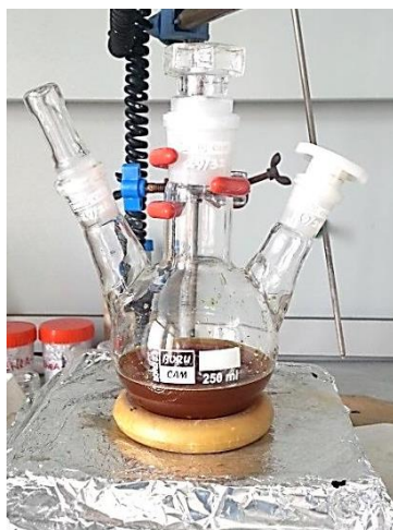
Figure 3.1 : Photograph shows synthesis of \text{Fe}_3\text{O}_4 nanoparticles inside the three-neck glass flask.
