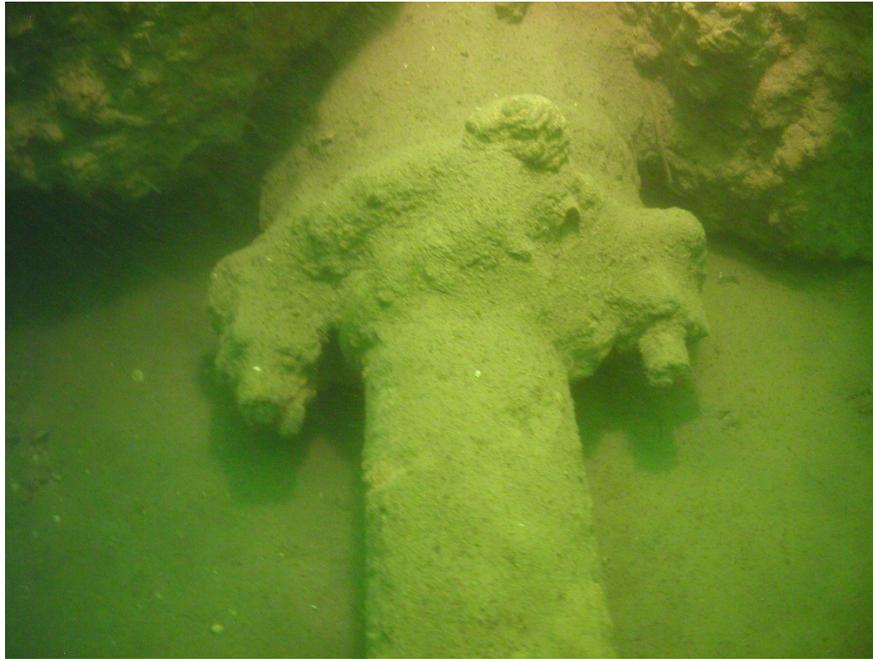
Figure 63: Piston with attached follower. (D. Van Zandt, 2009)
