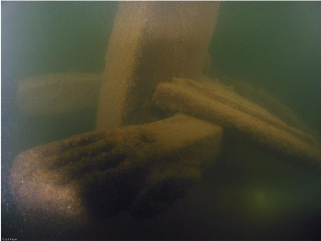
Figure 36: Port cathead with heart-shaped cleat. (J. Papes, 2007)
