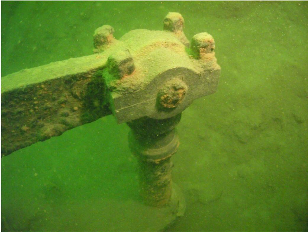
Figure 71: Valve lever pivot. (D. Van Zandt, 2009)
