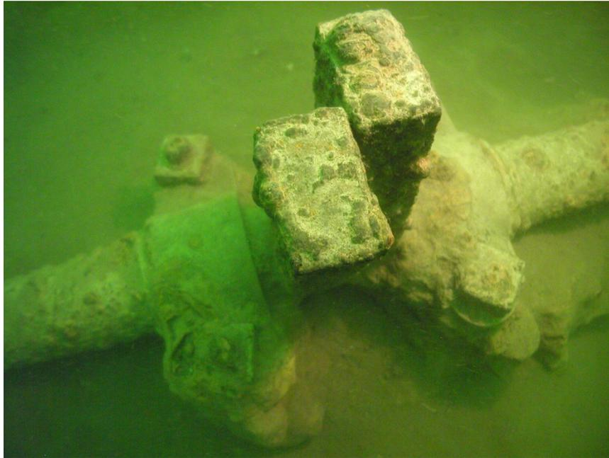
Figure 73: Rocker shaft alignment pins. (D. Van Zandt, 2009)
