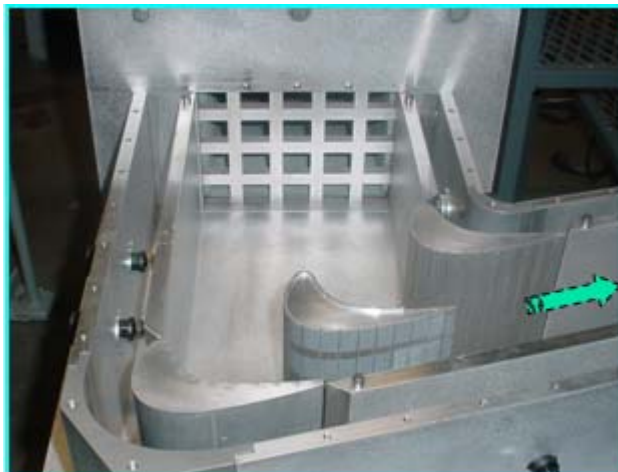
Fig. 4.5 Turbulence generating grid at the inlet of the test section
