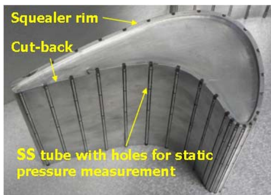
Fig. 4.6 (a) Test blade with surface pressure taps (b) Squealer rim blade tip
