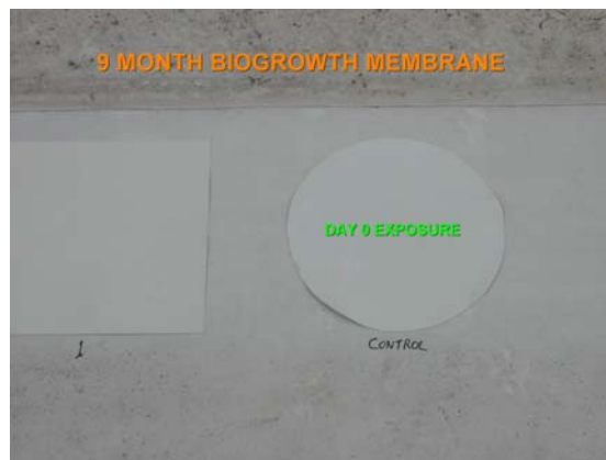
Figure 3. Experimental Installation in Homestead, FL. left: sample with photocatalytic coating; right: control; above: 9 months-aged inoculation membrane.
