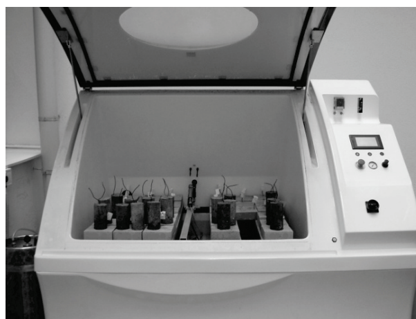
Figure 2 Specimens exposed to simulated marine environment in salt spray chamber
