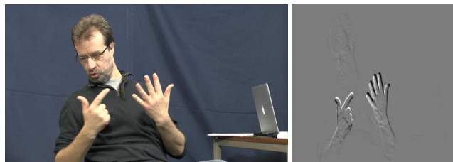
Figure 1. Left : Original RGB-data. Right : Model input. The RGB channels are converted to gray-scale, resized to 128x128 pixels and the previous frame is subtracted from the current frame to remove static information.
