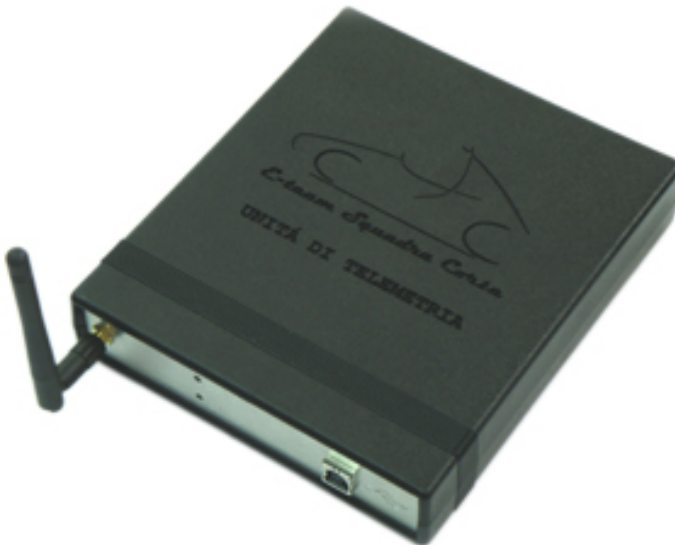
Figure 10.4: The ET3 telemetry units
