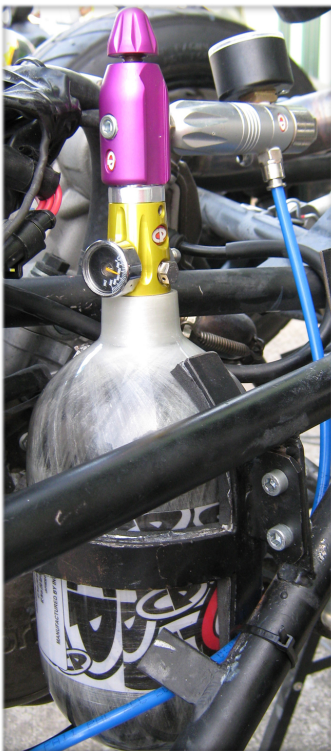
Figure 9.3: The pneumatic system – air tank with low pressure regulator and double-effect cylinder mounted on the gear lever
