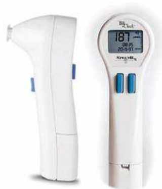
Figure 1-17: Non-invasive Bilirubin detector based on MOEMS spectrometer.
