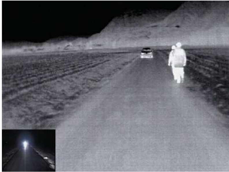
Figure 1-18: Using an IR sensor it is possible to detect people otherwise not visible at night.
