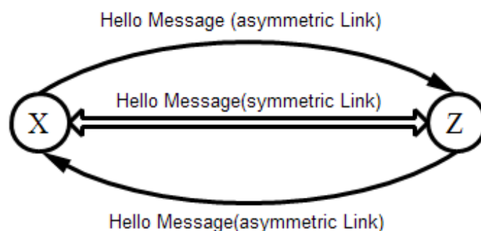
Figure 3.8 OLSR symmetric link formation (Hello Message Exchange)
