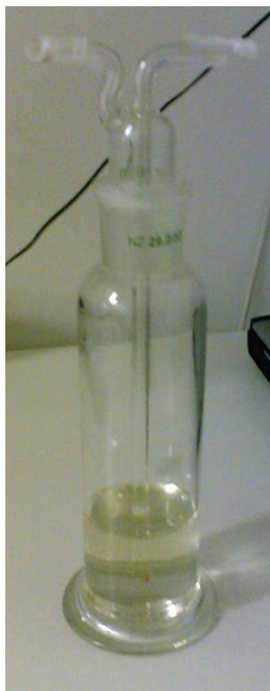
Figure 92. Picture of the bottle collecting condensed water vapor coming out the cathode side of the AMFC used for subsequent measurement cycles reported on Figure 90
