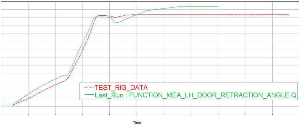
Figure 3. 26 – Tuning of door actuator seal friction
