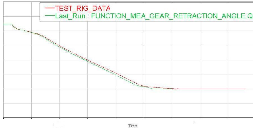
Figure 3. 27 – Tuning of gear actuator seal friction
