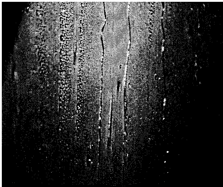
Figure 4.4: Picture of the COPAIN condensing plate during a test at high mass transfer rate and high velocity
